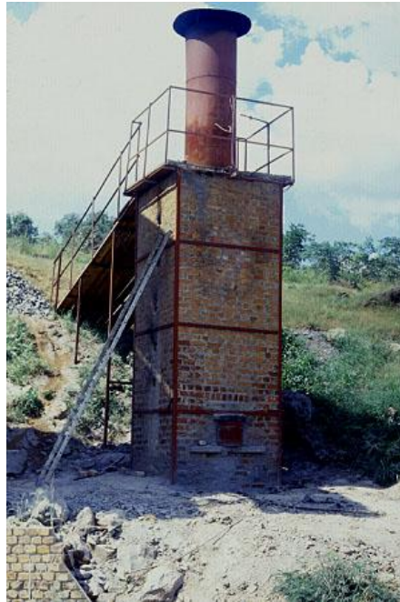
Figure 2: A vertical shaft kiln for small-scale production of lime. Chegutu, Zimbabwe. Photo: Practical Action / Kelvin Mason.
