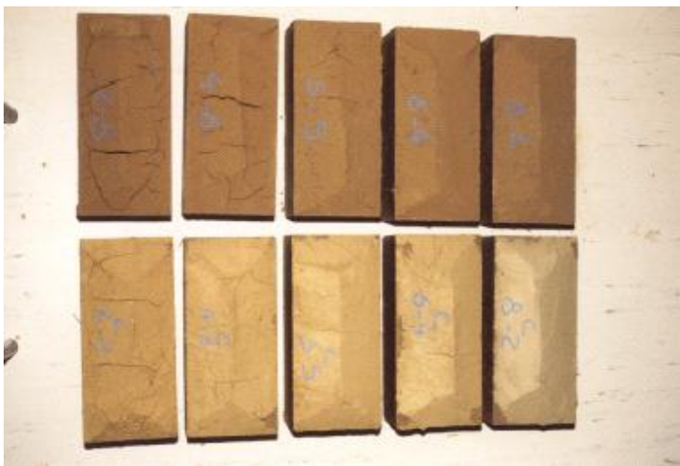
Figure 3: Test carried out on unstabilised and stabilised mortars to determine the optimum soil/sand ratio. Photo: CRATerre/EAG
