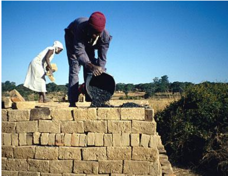
Figure 1: Boiler waste is sieved and used as a fuel for firing brick clamp kilns at Kurewasekwa Cooperative in Epworth, Harare. Photo: Practical Action / T. Schilderman
