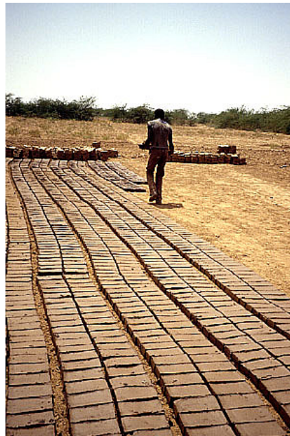
Figure 1: Moulded bricks pre-drying in the sun before being fired near Kassala. Photo: Theo Schilderman / Practical Action.
