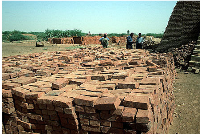
Figure 3: Pile of clay fired bricks with scotch kiln behind. Photo: Mohammed Majzoub / Practical Action.
