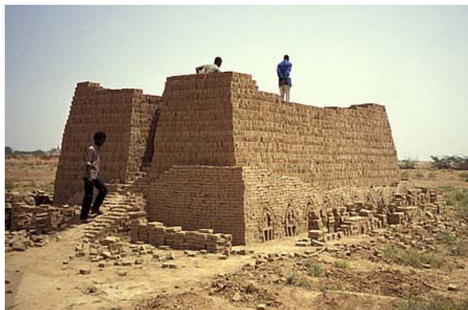
Figure 2: A brick clamp kiln is shown near Kassala. Photo: Theo Schilderman / Practical Action.
