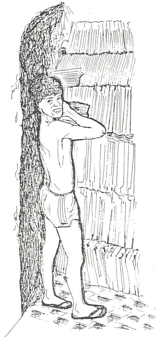
Figure 30: Stacking the tiles in the kiln.
