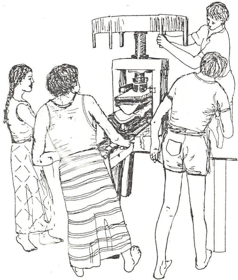
Figure 24: Pulling the lower die from the press.
