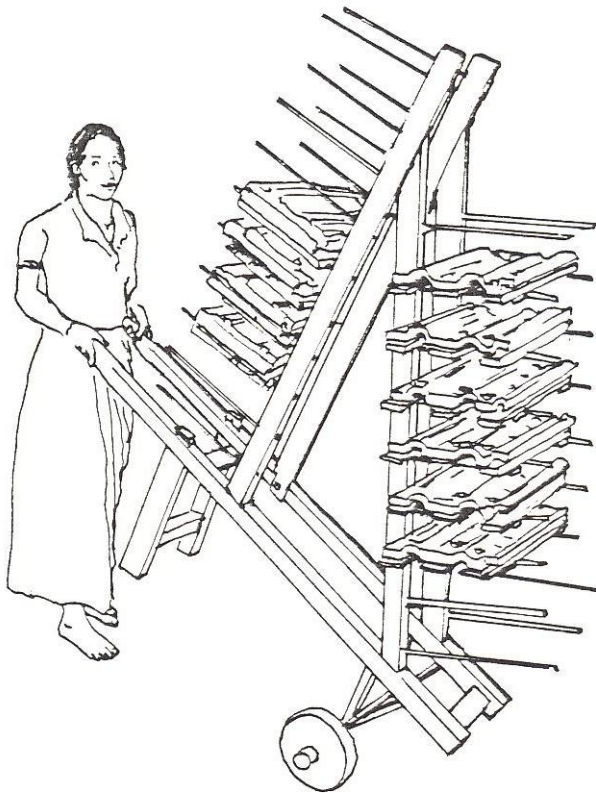
Figure 5: A cart for moving wet tiles.
