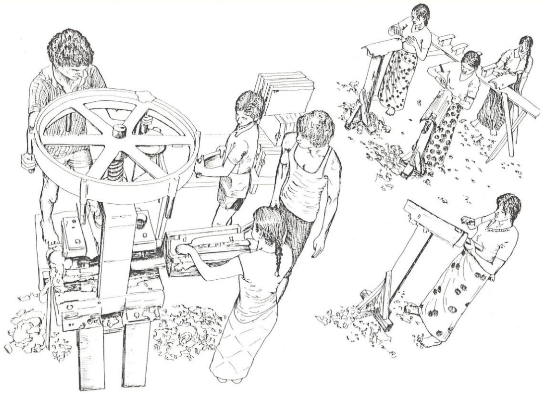
Figure 27: An overview of a single action press production site.
