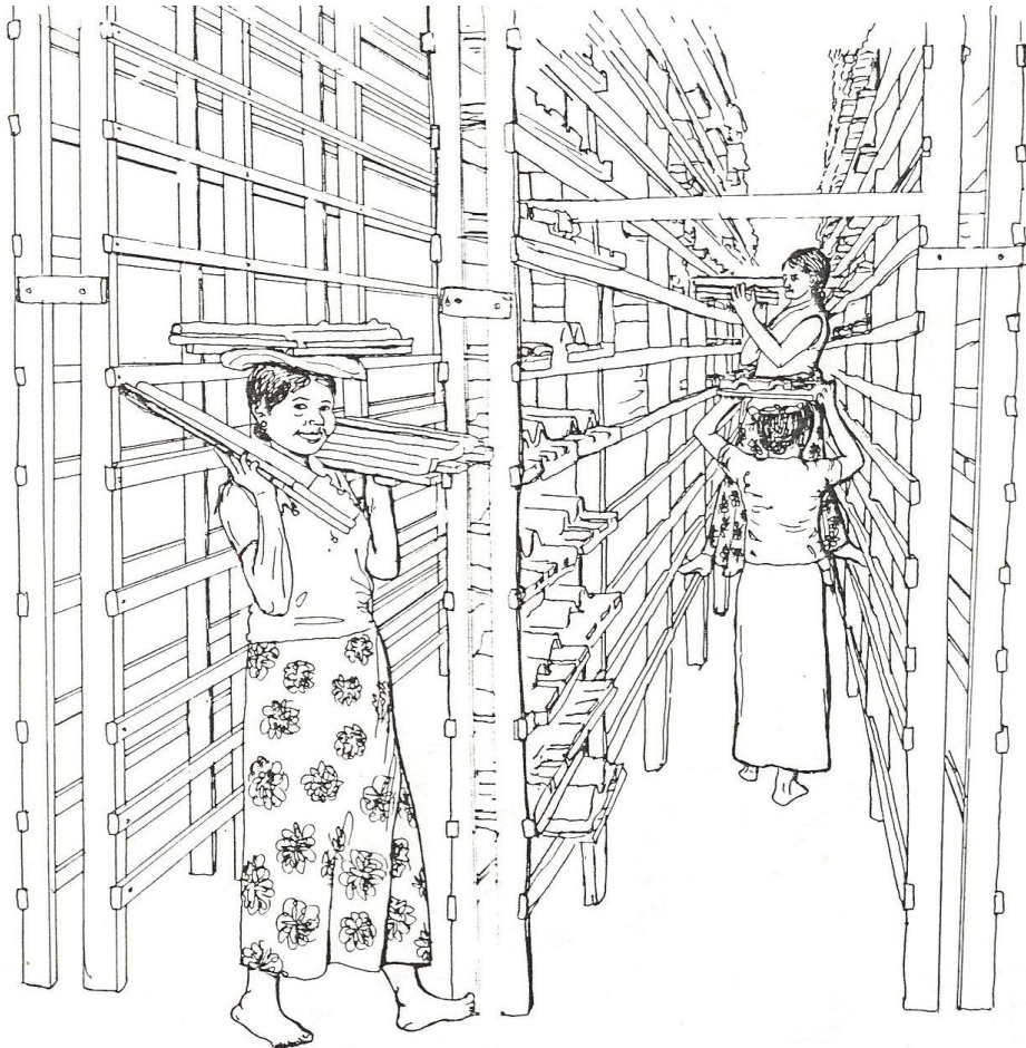
Figure 28: Carrying and stacking wet tiles on the racks.
