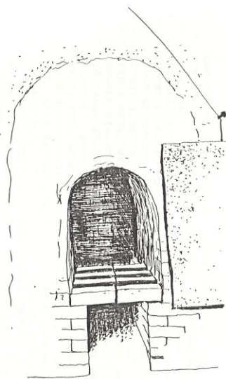
Figure 10: Kiln firebox fitted with butting brick grate arches.
