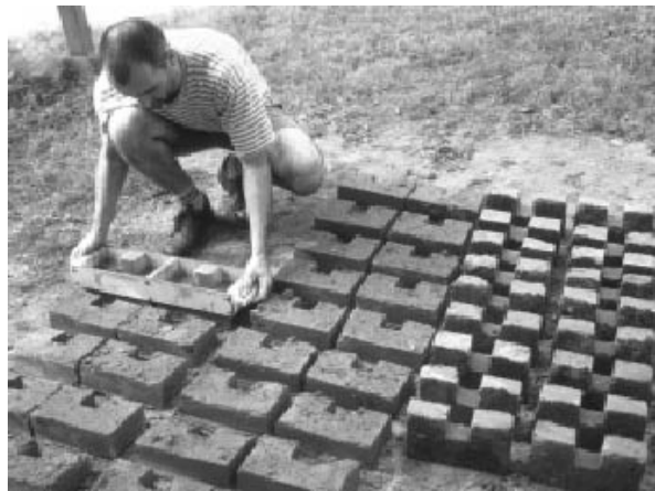
15-6 Production of special adobes
