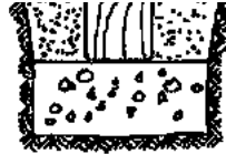
POST ON CONCRETE FOOTING
