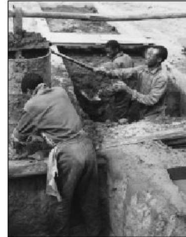
Fig 4: Filling a pugmill with clay.
