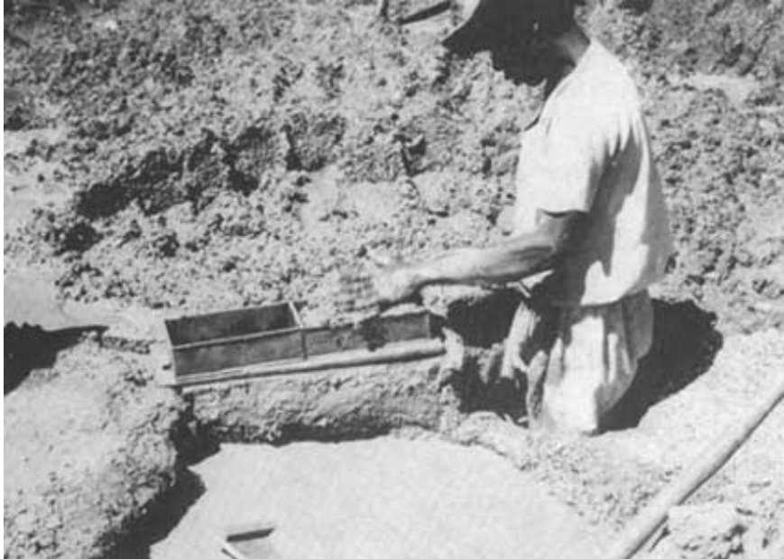
Figure V.6 - Slop-moulding in double cavity metal mould, with moulder standing in deep hole (West Sudan)
