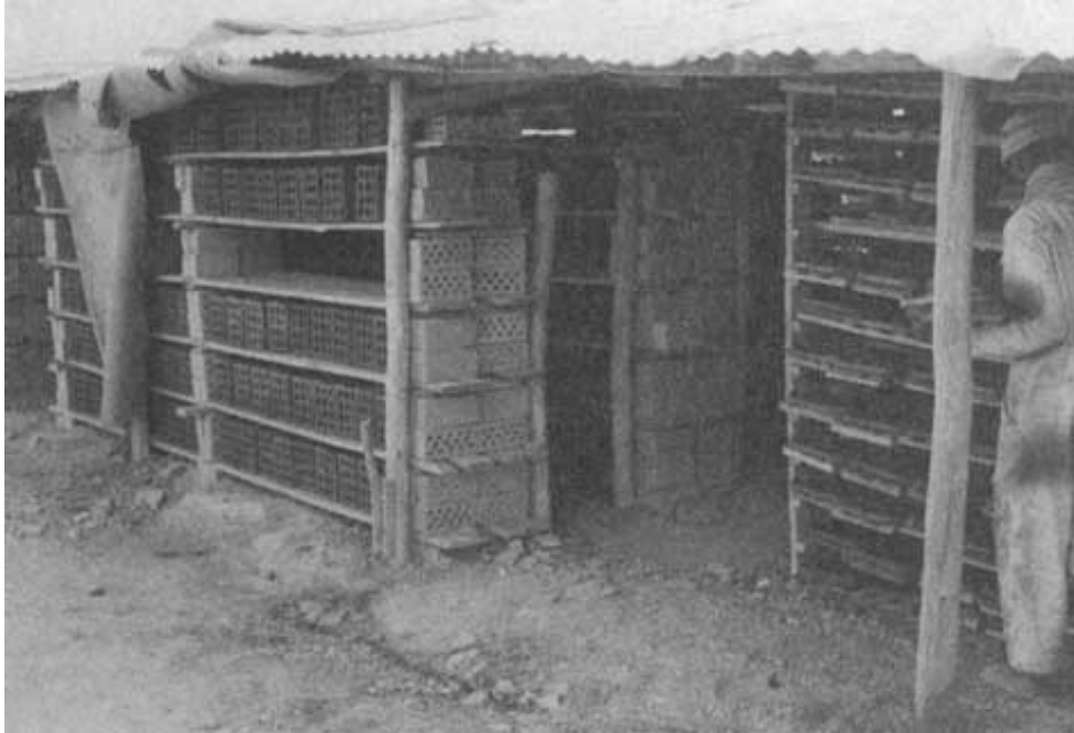
Figure VI.11 - Rack-drying under cover, with removeable side screens (Madagascar)
