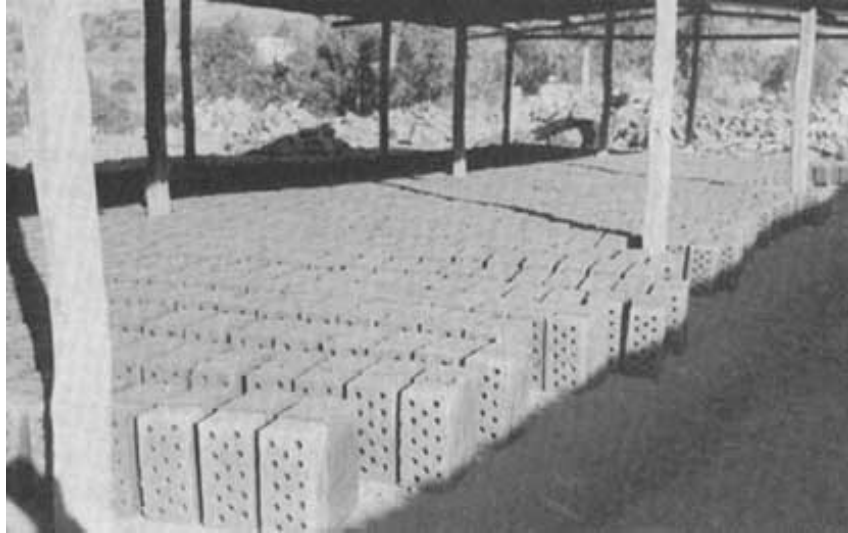
Figure VI.9 - Open-sided drying shed (Madagascar)
