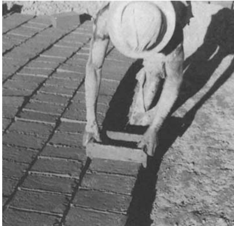
Figure VI.2 - Bumpy drying ground covered with debris (Madagascar)
