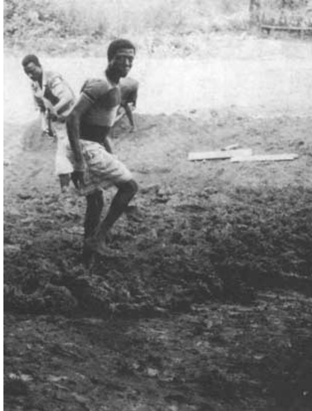
Figure IV.13 - Foot-treading clay on concrete floor (Ghana)
