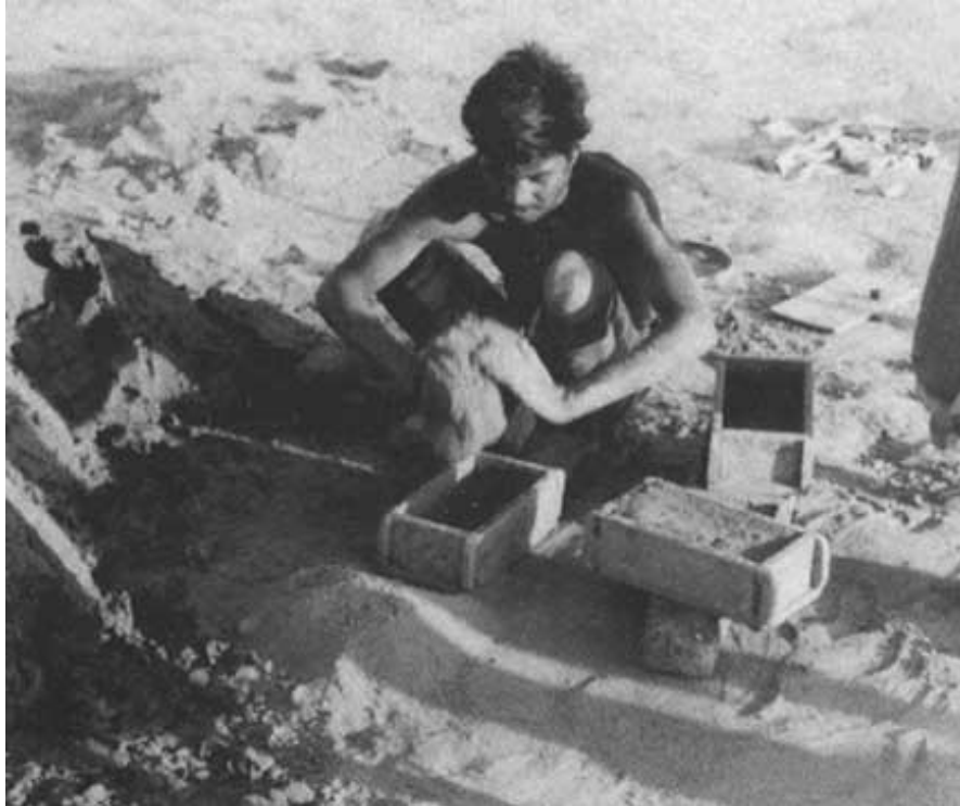
Figure V.10 - Moulder using sand to prevent sticking (India)
