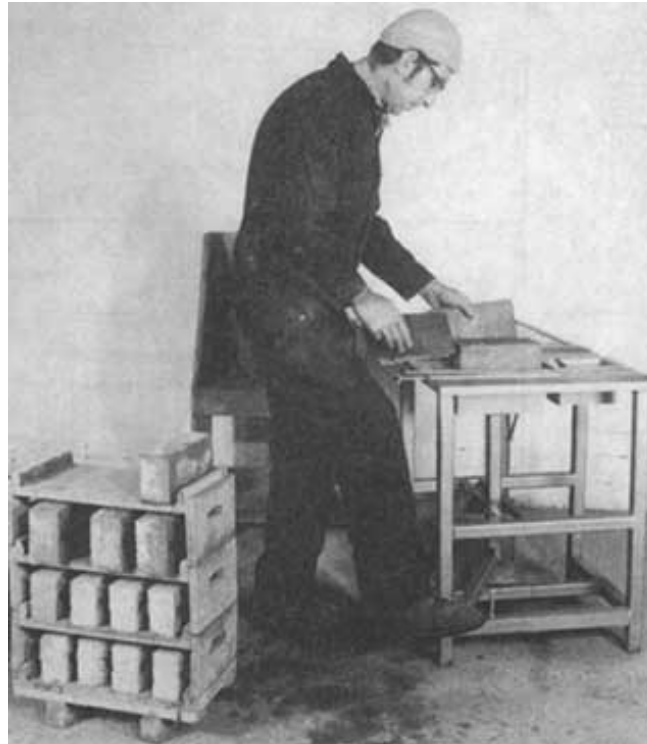
Figure V.18 - Table mould; pedal being depressed to eject brick. Each brick is handled with pallets and stacked on racks (United Kingdom)
