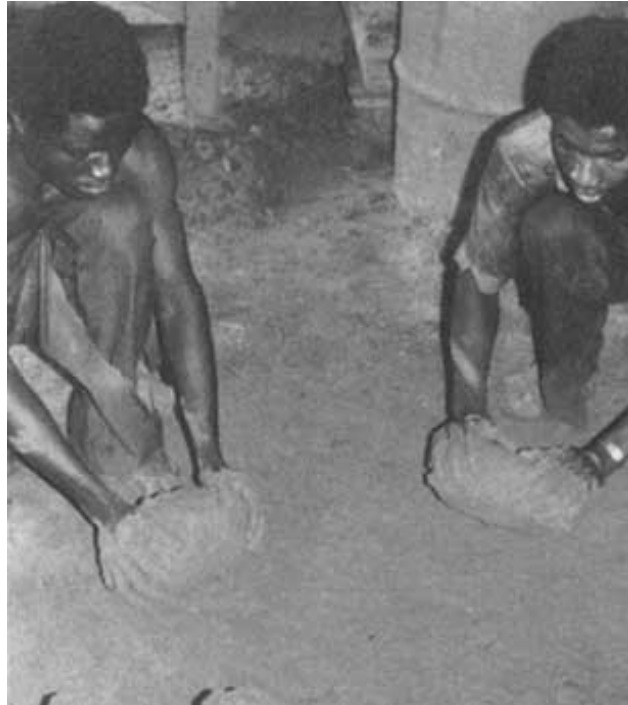
Figure V.12 - Clot-makers rolling clay in sand (Ghana)
