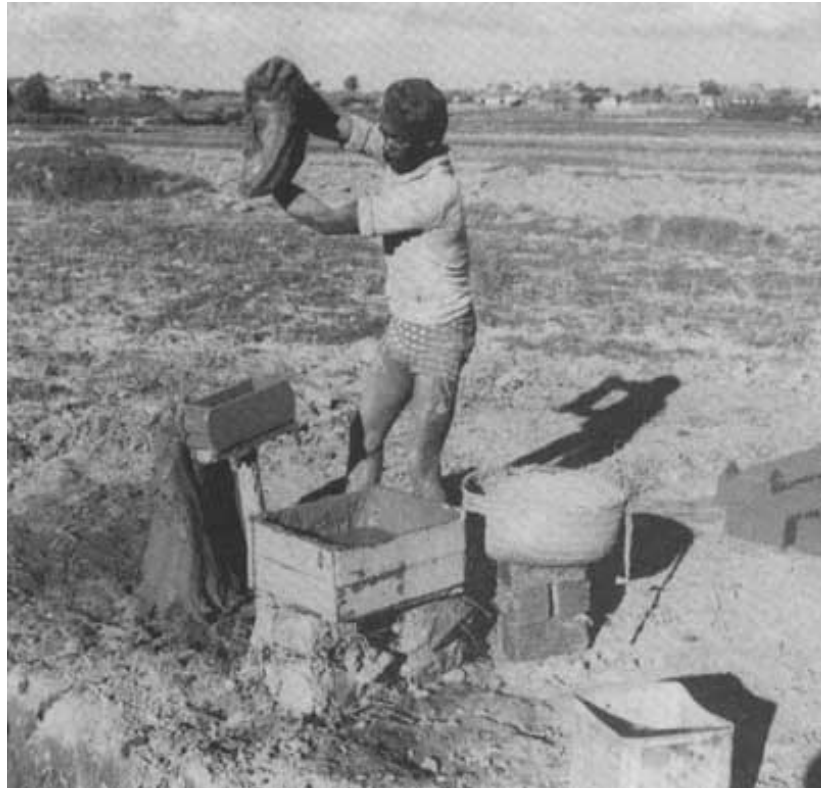
Figure V.8 - Moulding with sand-covered mould base (Madagascar)
