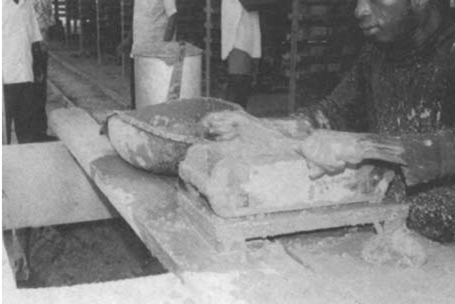
Figure V.7 - Striking off excess clay in slop-moulding (Ghana)
