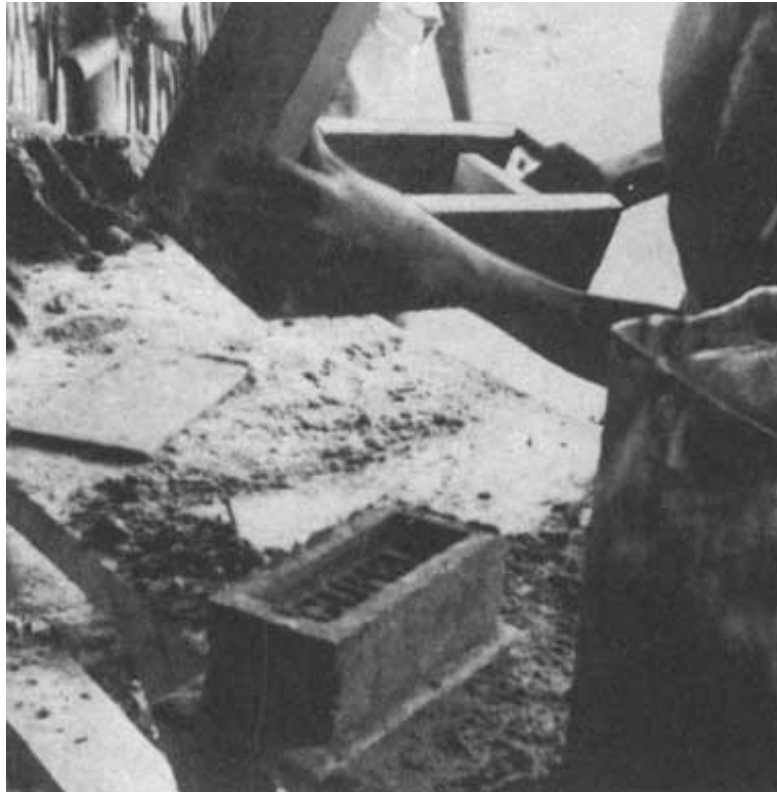
Figure V.13 - Hinged-bottom mould and moulded brick (Southern Sudan)
