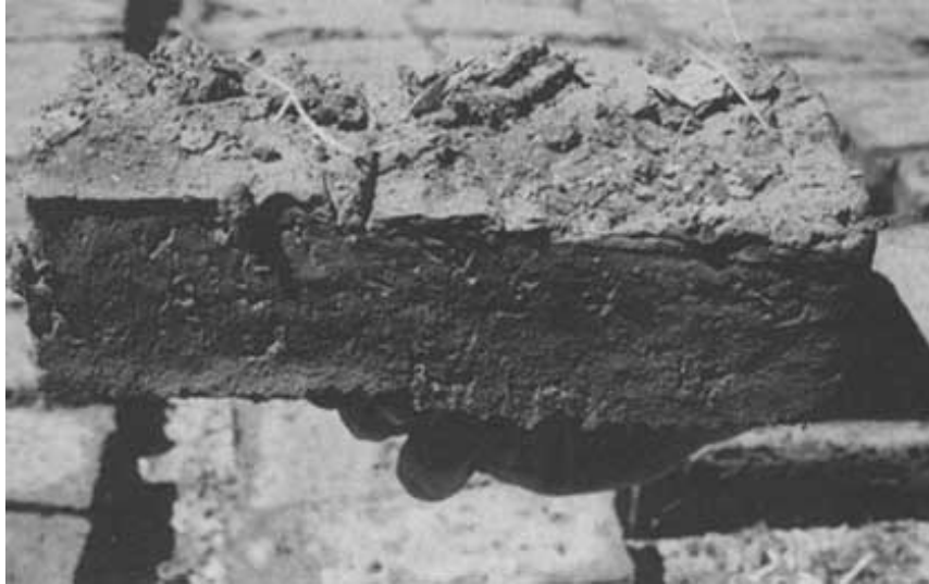
Figure VI.3 - Partly dried brick distorted and covered with debris (West Sudan)
