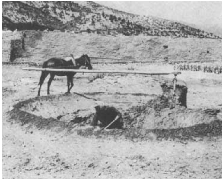
Figure IV.12 - Animal-powered pug mill (Turkey)
