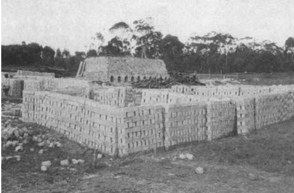
Figure VI.5 - Drying being completed in hacks (Madagascar)
