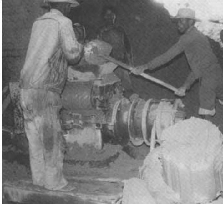
Figure IV.10 - Motor-driven pug mill (Madagascar)
