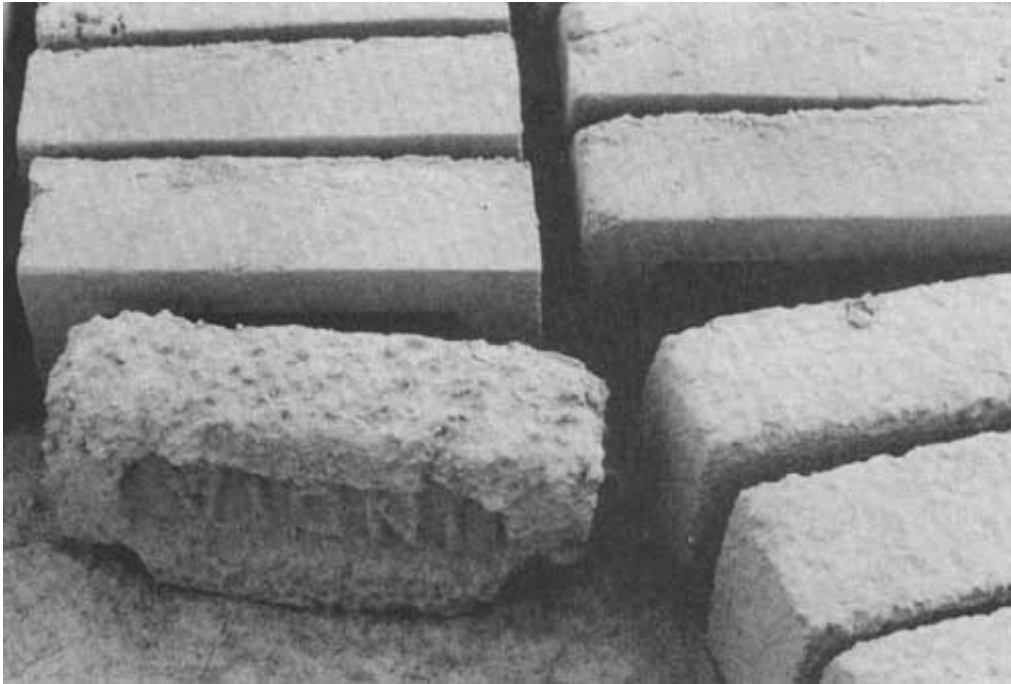
Figure VI.6 - Rain damage to green bricks - No damage on protected bricks
