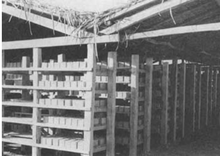
Figure VI.10 - Rack-drying under cover (Madagascar)
