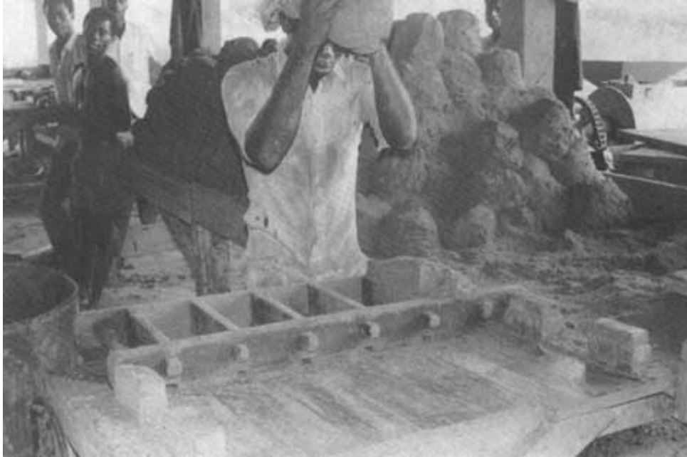
Figure V.14 - Moulder throws preformed clot. Use of five cavities mould (Ghana)
