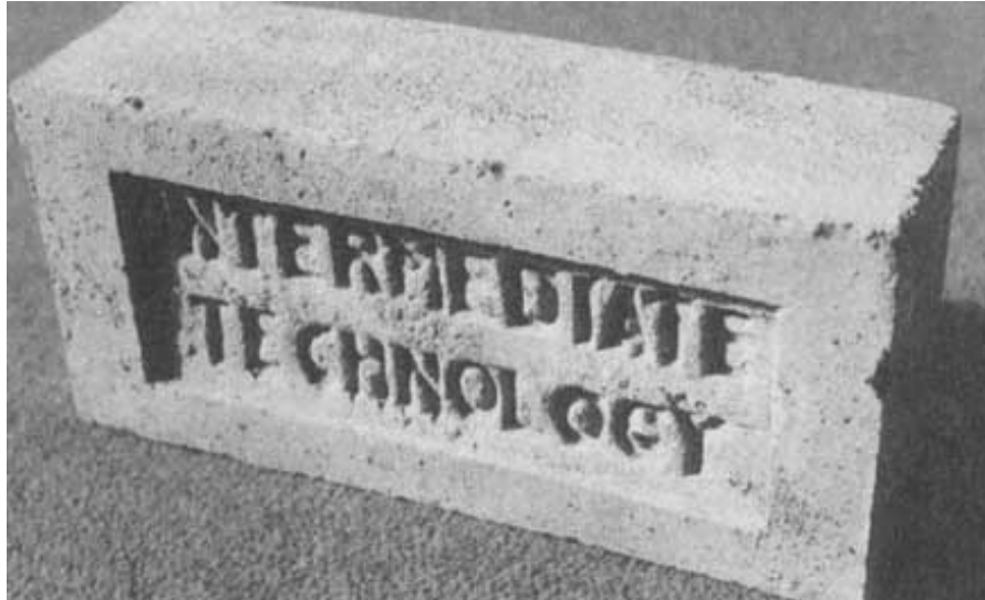
Figure V.21 - Brick moulded in hinged-bottom mould by
