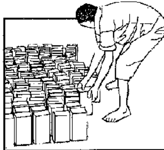
Placing the brick on its end.
