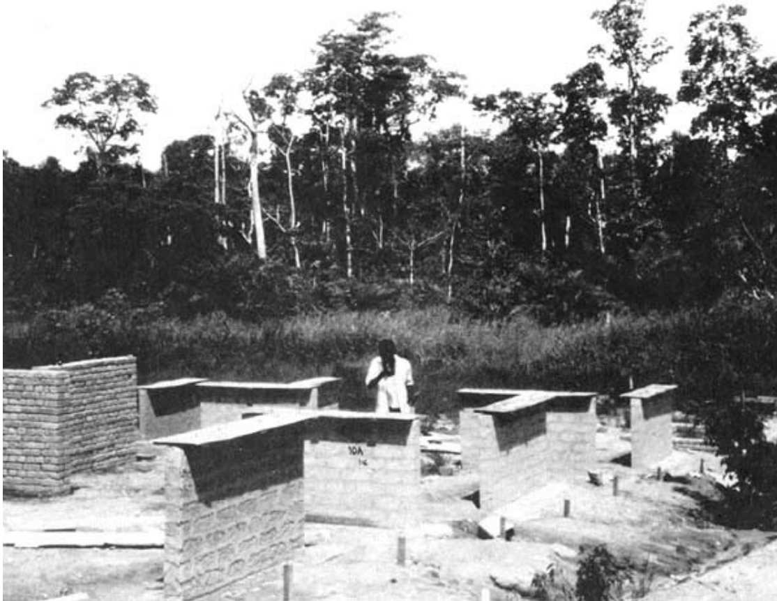
Figure V.11. Exposure site in Ghana where soil block are being weathered
