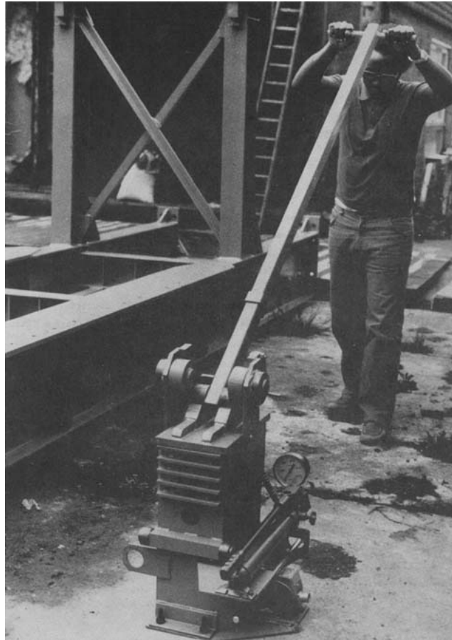
Figure IV.12. The Brepak machine
