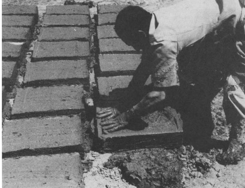
Figure IV.4. Adobe block manufacture
