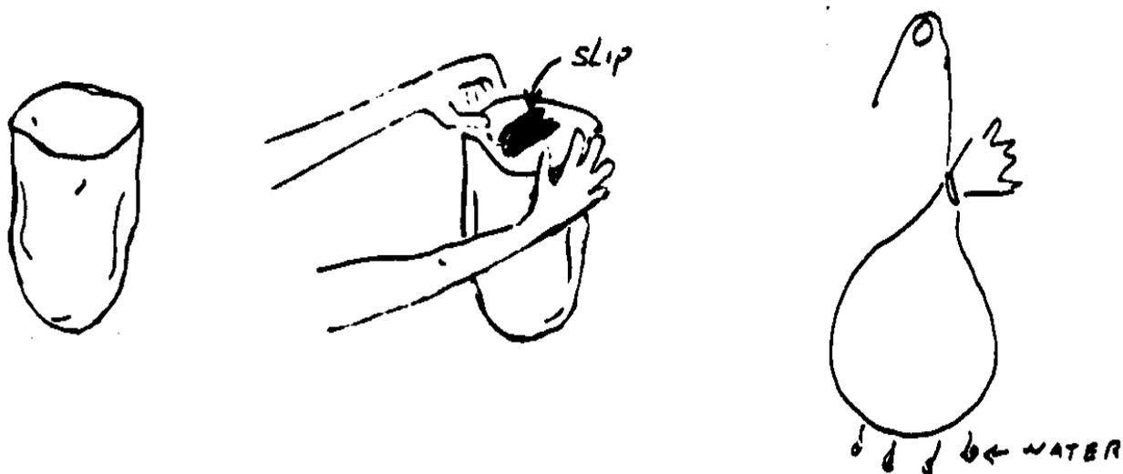
**Figure 20. Drying Clay in a Cloth Bag**
