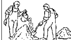
Turn the pile of wet soil a second time, continuing to water if necessary.
