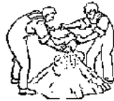
Pour out the dry materials (earth, sand, gravel, cement).
