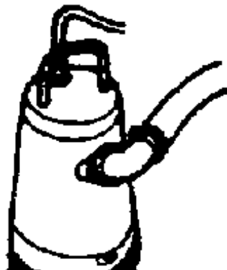
E. Mobile centrifugal pump
