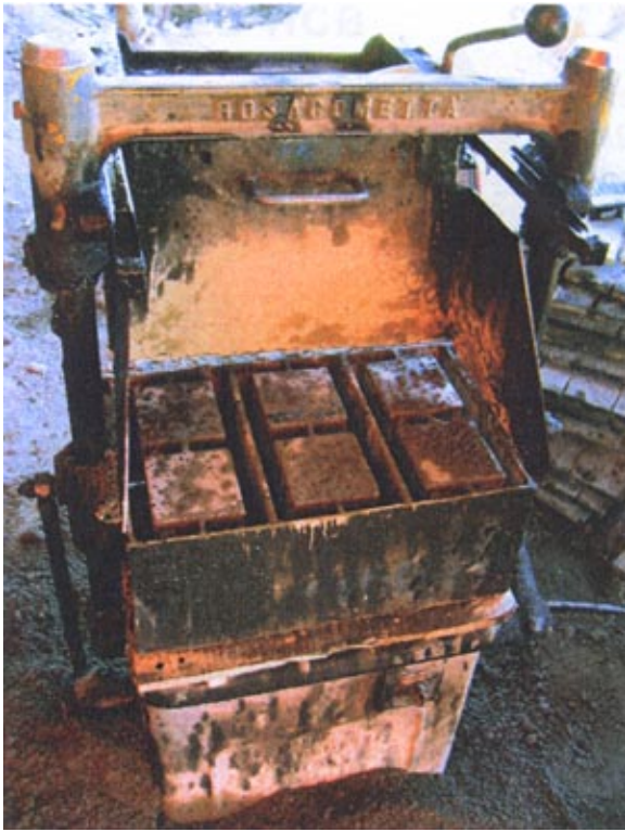
The machine used for the production of HCBs
