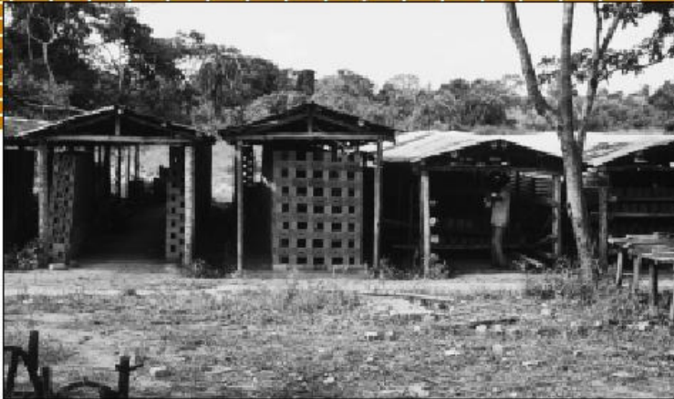
Fig. 8: Rack drying under cover: moderate drying conditions for perforated bricks
