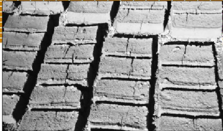
Fig. 5: Wrong drying process: green bricks are exposed to sun and wind, cracks develop on the surface
