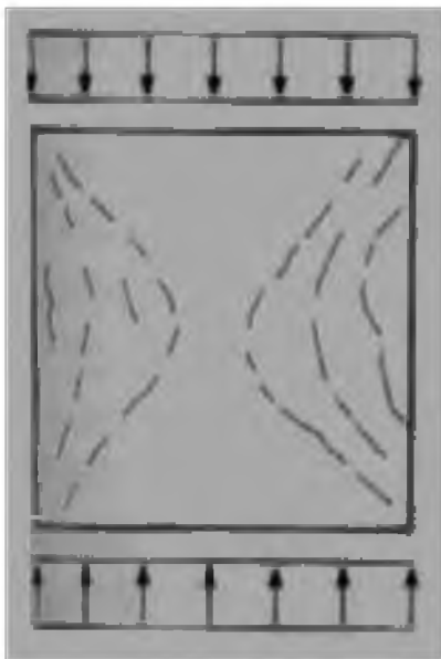
Figure 5.2a: Cracking Pattern Of a Cube
