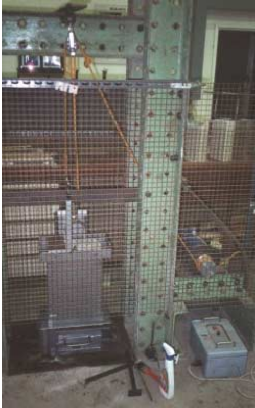
Original test rig (cement impactor)
