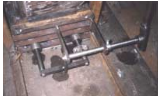
Ejection mechanism added
