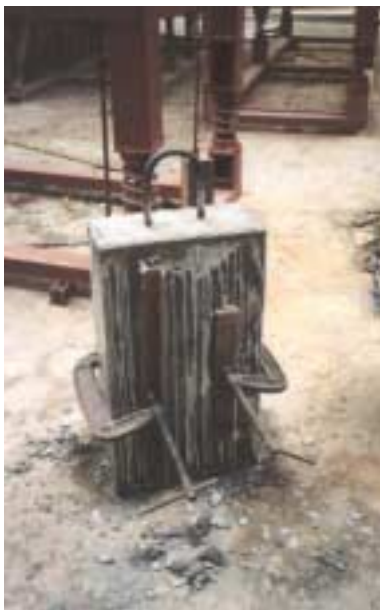
New cast concrete impactor
