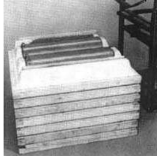
Semi-sheet moulds stacked to set overnight.
