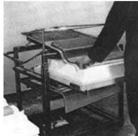
Placing wet Semi-sheet on the setting mould.
