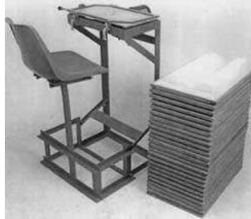
The TARA Vibrator with a stack of moulds
