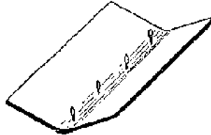
Fig. 12 Ridge tile with cast-In wire loops
