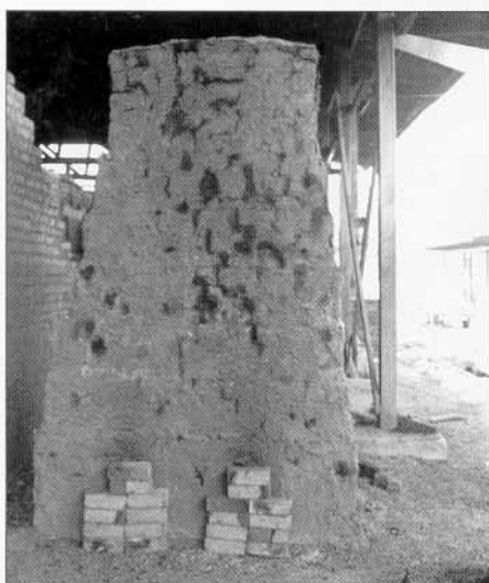
Figure 1 Small scale factory using clamp firing with firewood
