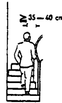
If stairs are narrow or curved, distance of walk line from outer string is 350-400 mm (14-16 in)
