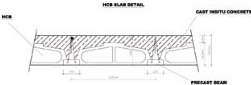
Fig-4s section of slab at final condition
