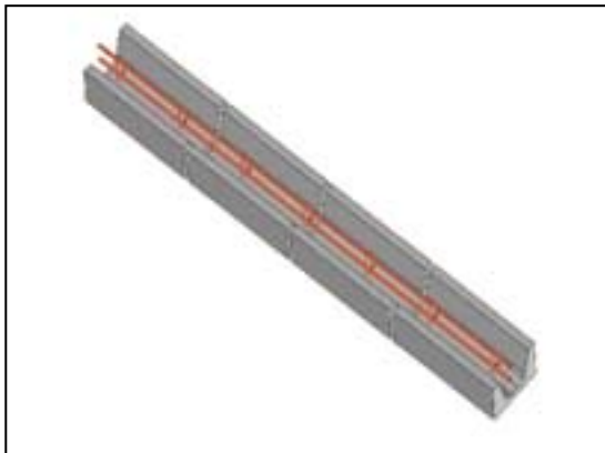
4 U-shaped HCBs joined together as a lintel with reinforcement
