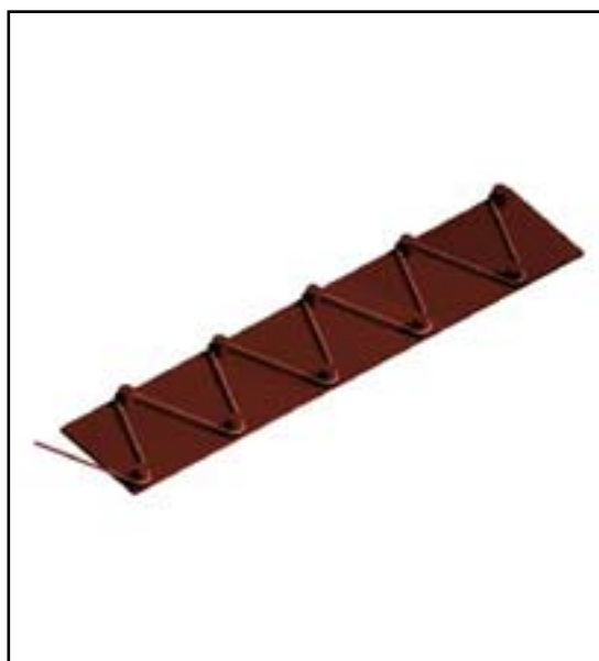
Model of the formwork with ready-bent stirrup on it
