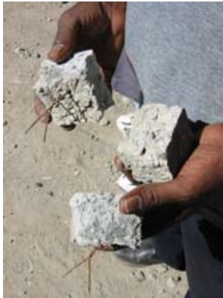
The concrete spacers with wires for fixing them
