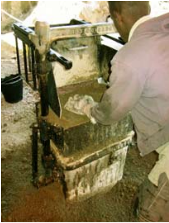
Concrete is filled up during compacting until the molde is filled
