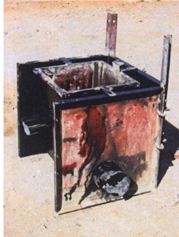
The mould viewed from the side of the catch drain (front panel removed)
