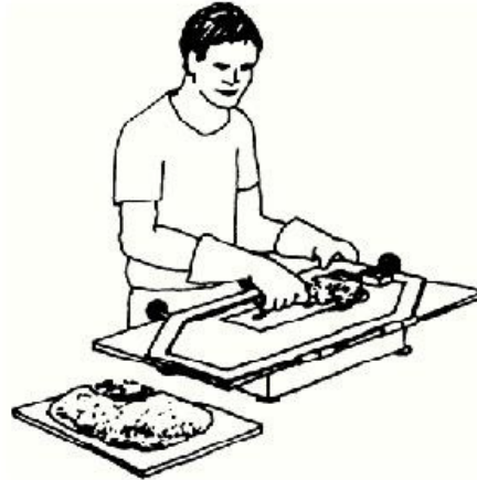
Figure 2: Work the mortar mix under vibration
