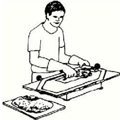
Figure 3: Smooth under vibration
