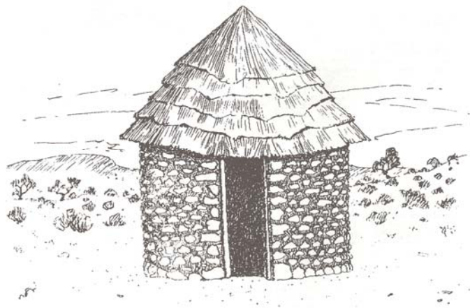
Figure 1: A rondavel built of earth and stone
