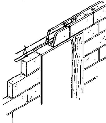
**Figure 43: Channel form block in a tie-beam configuration**
