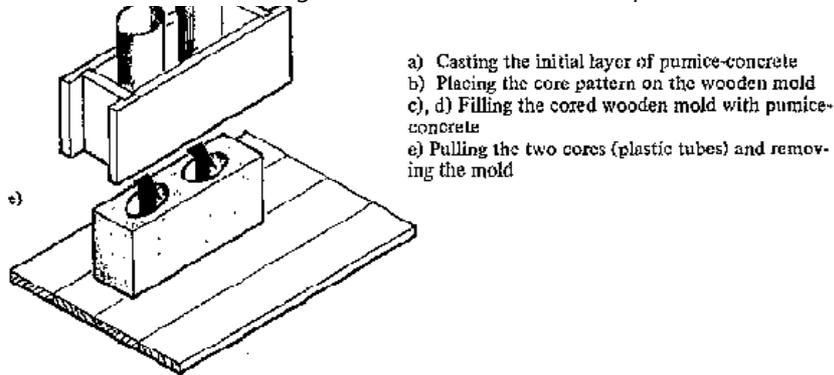
**Figure 33: Forming pumice-concrete two-cavity blocks**
