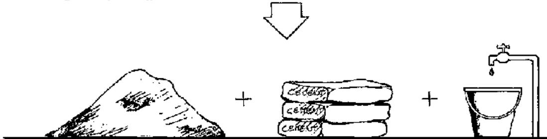
c) Materials for pumice concrete: pumice gravel, cement, water
