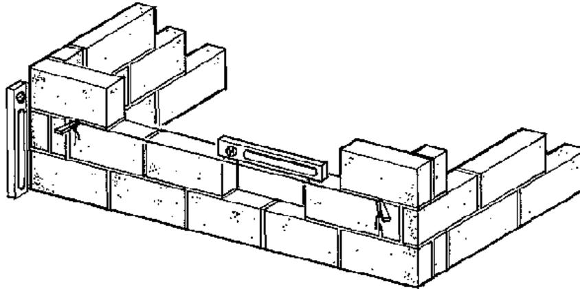
**Figure 57: Setting up brick walls**
