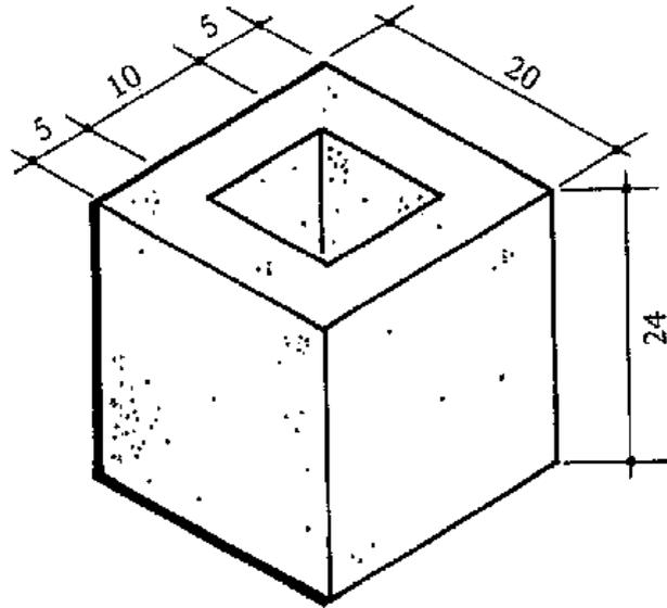
**Figure 44: Chimney block**
