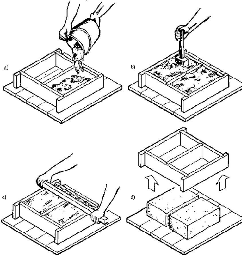
a)-c): Manual compaction of pumice-concrete in the mold
