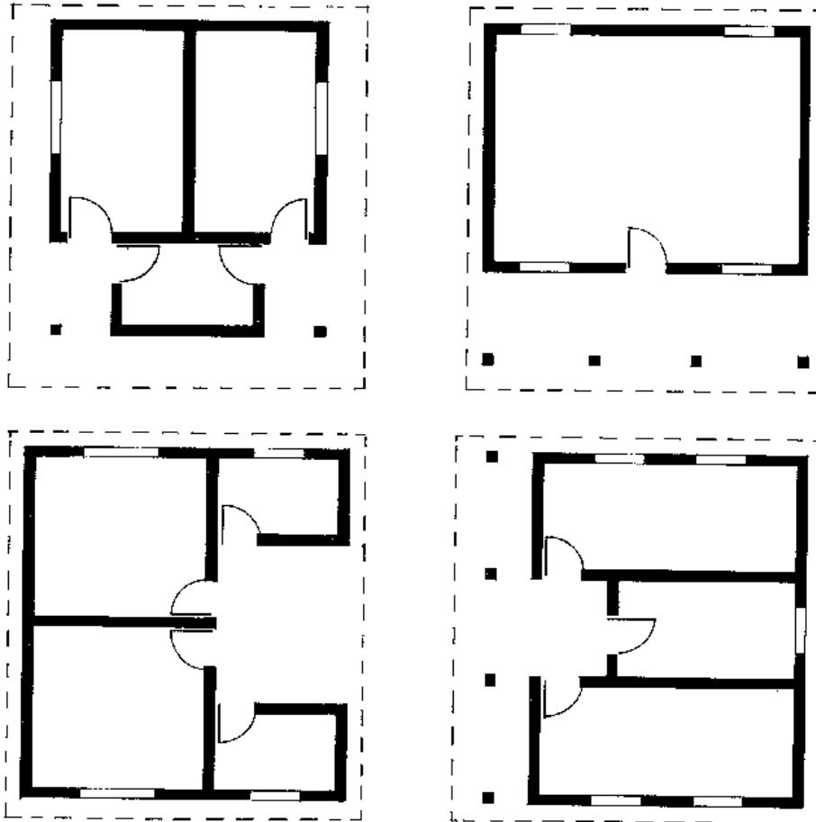
**Figure 18: Selection of four 30 m<sup>2</sup> plans**
