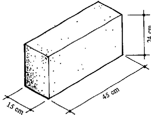
**Figure 27: Pumice-concrete solid brick.**
