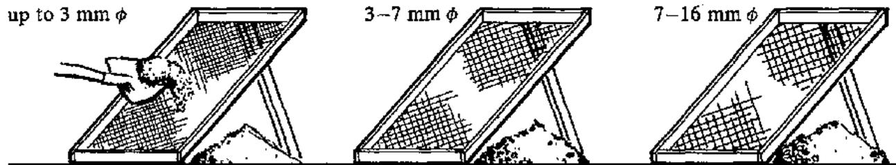
**Figure 23: Screening the raw material**
