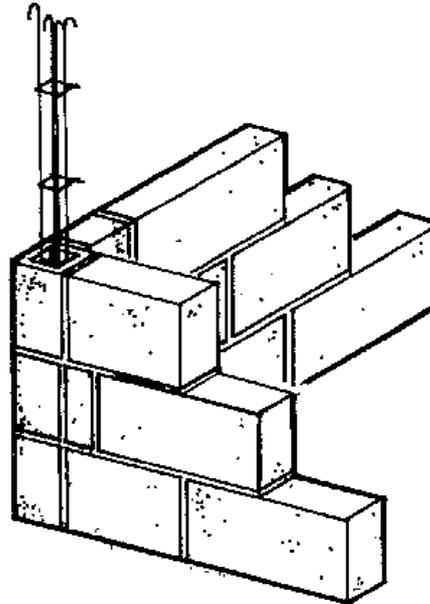
**Figure 45: Masonry corner with channel block serving as support framework**
