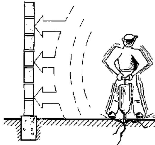
Fig. 10b: Pumice is sound-absorbent
