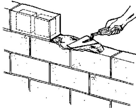
**Figure 32: Spreading mortar on a cavity block**
