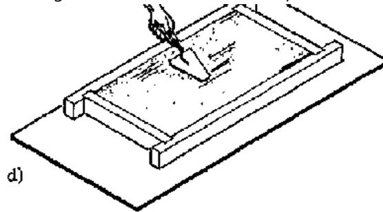
Fig. 38: Forming pumice-concrete panels
