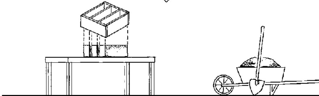
e) Filling and removing of the molds
