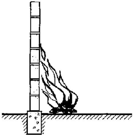
Fig. 9b: Pumice is refractory
