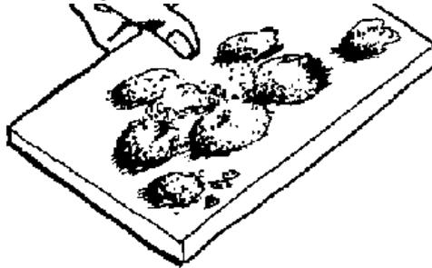
**Figure 21: Proper moisture content of pumice-concrete**
