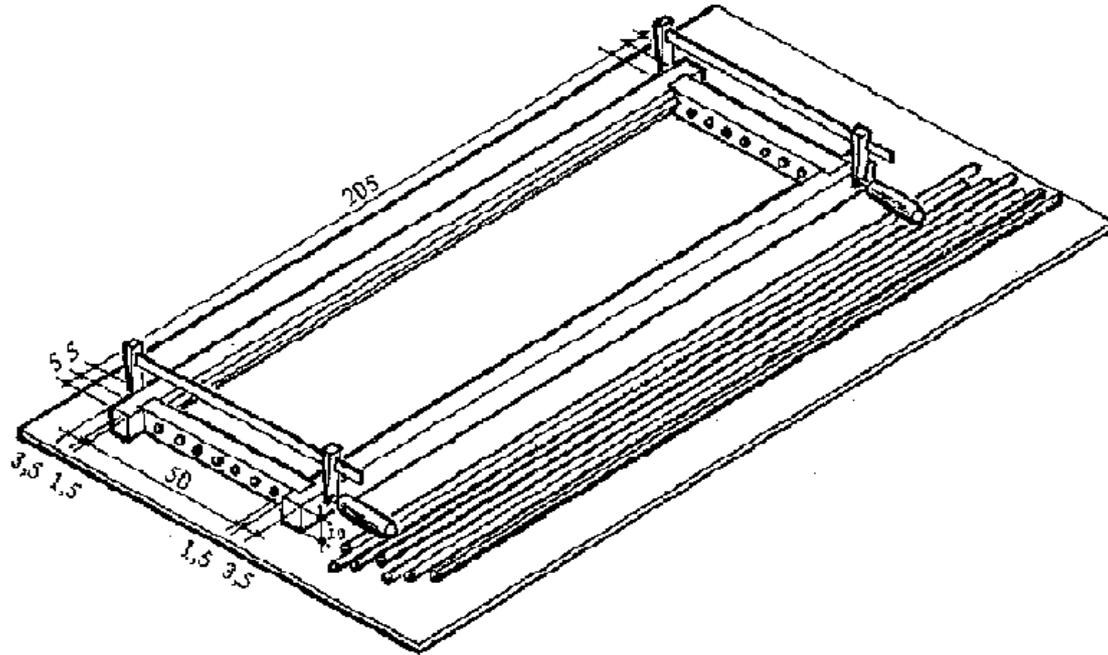
**Figure 39: Mold for hollow-core planks**
