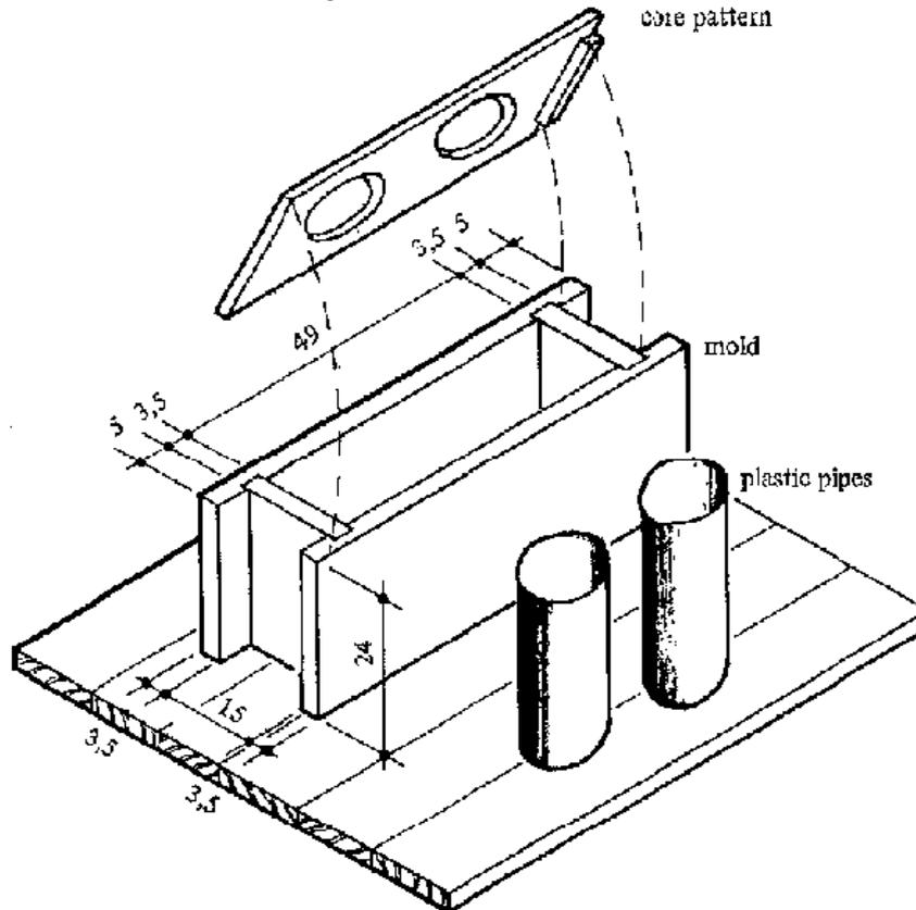
**Figure 31: Wooden mold for two-cavity blocks**
