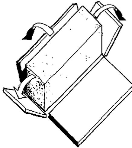
**Figure 26: Immediate removal of forms possible**
