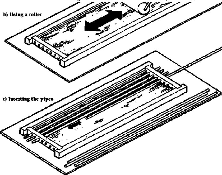
**Figure 40: Forming pumice-concrete hollow-core planks**
