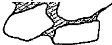
Fig. 2a: HARDENED CEMENT PASTE BINDS STONES TOGETHER AND FORMS A SOLID MASS
