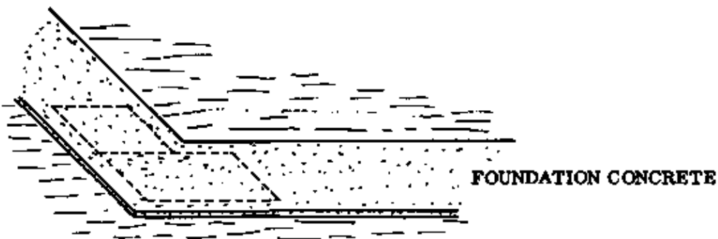
Fig. 3 SETTING OUT THE FOOTINGS (ENLARGED DETAIL)
