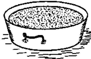
Fig. 1: FILL HEADPAN HALF FULL AND SMOOTH THE SURFACE
