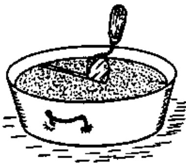
Fig. 2: MAKE A CUT WITH THE TROWEL
