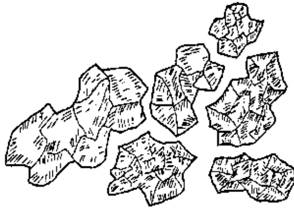
Fig. 2: SHARP SAND (ROUGH SURFACE)
