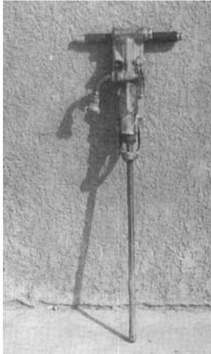
Rock drill with drill bit \phi 34 mm, length 800 mm
