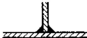
Welding in cross-section
