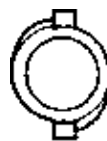
16. Dog Clutch for quick connection of two pipes or hoses with dog clutches by a quarter turn, e.g. for fire brigade.
