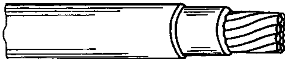
Figure 2 Plastic cable, double-insulation, multi-wire, (Cu – NYY 1 x 50 mm 2 , Al-NAYY 1 x 50 mm 2 )
