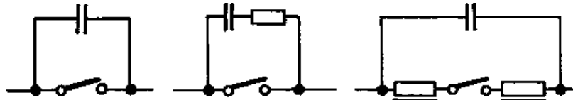
Interference suppression of switch gears
