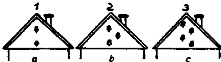
Fig. 2.30. Arrangement of insulators at buildings
