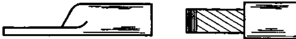
Fig. 3.22. Entering the conductor into the cable terminal's barrel by means of a wire binding
