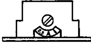
Fig. 7.12. Setting the thermal overcurrent release at the motor protection switch
