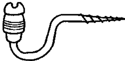
Fig. 2.7. Insulator with swan-neck spindle
