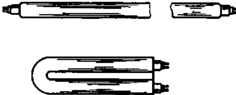
Fig. 5.35. Straight and U-shaped fluorescent lamp
