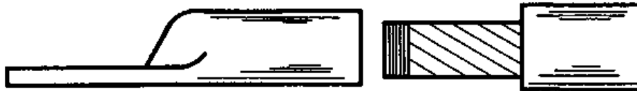
Fig. 3.22. Entering the conductor into the cable terminals barrel by means of a wire binding
