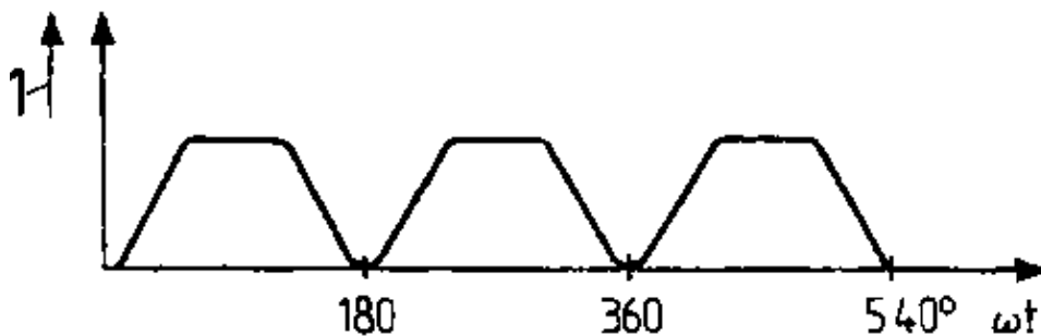
Figure 91 Torque of a conductor loop in dependence on the rotational angle
