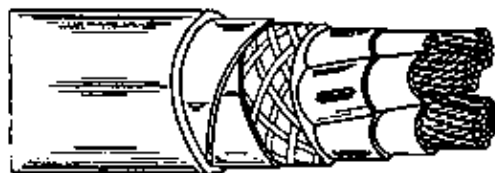
Figure 5 Strong rubber hose cable
