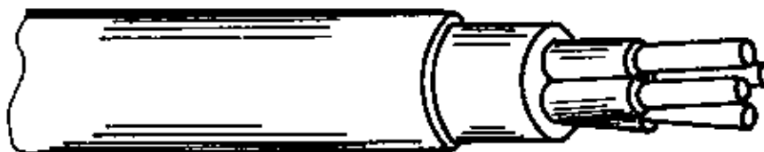
Figure 3 Plastic cable, multiple insulation, multi-core, single-wire, (Cu – NYY-I 4 x 2.5 mm 2 re, Al – NAYY-I 4 x 2.5 mm 2 re)
