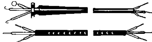
Figure 30. Interconnection line with fixed connection at both ends - 1 with integral appliance lead-in, 2 with outer braiding
