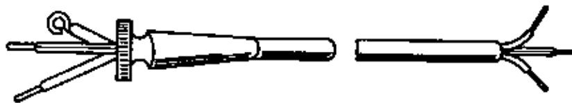
Figure 2 Light rubber hose cable (ready-made cable)
