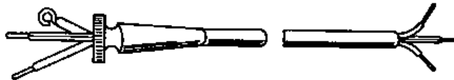
Figure 2 Light rubber hose cable (ready-made cable)
