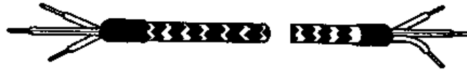
Figure 3 Light rubber hose cable with yarn wrapping (ready-made cable)
