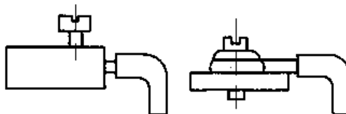
Figure 22 Connection points with correctly removed core insulation
