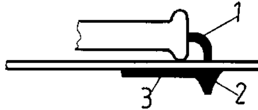
Figure 11 - Components and printed circuit boards - 1 lead, 2 soldering point, 3 printed circuit board trace
