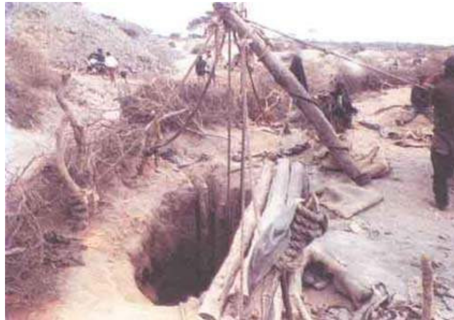
Figure 11: Artisanal Hoisting Mechanism at Merelani Tanzanite Mines
