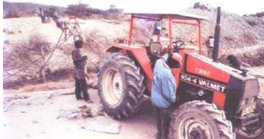
Figure 12: Artisanal Hoisting Mechanism at Merelani Tanzanite Mines
