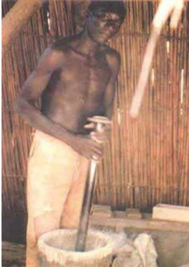
Figure 4: Crushing and Grinding of Ore Using the Jack Hammer
