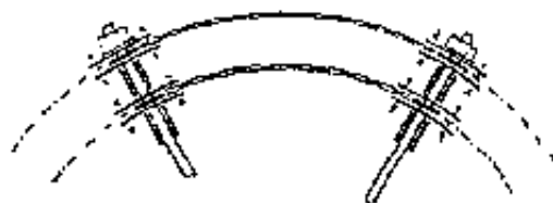
Fig.: Construction for inserting screen plates into a concentric drum. Source: Treptow.
