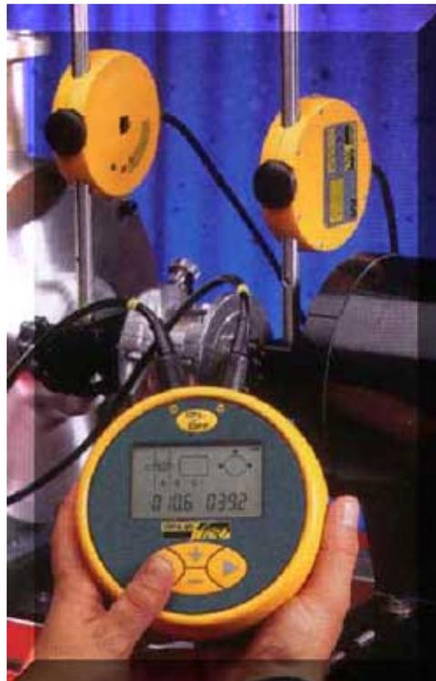
**LASER BASED SHAFT ALIGNMENT TOOL**
