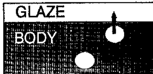
a) Section of glaze and body with two air holes. The one close to the surface rises.
