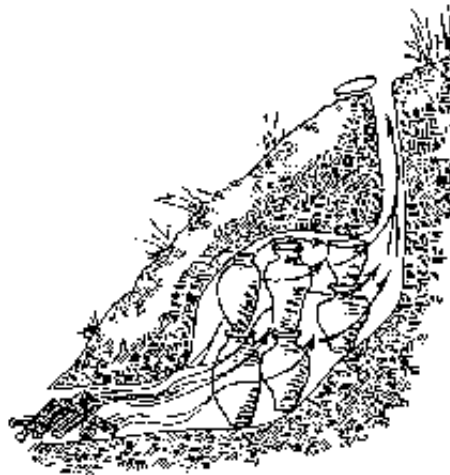
Fig.2-25: Cave kiln dug out of a clay bank.
