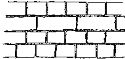
Fig.2-80: Mortar is used for filling the spaces between irregularity shaped bricks.
