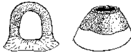
Fig.2-137: Two examples of glazed test pieces: a ring of clay and a cup with its bottom pierced.
