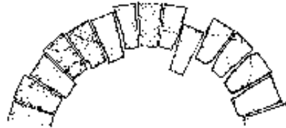
Fig.2-110: Look out for bricks falling in and refill mortar in loose joints.
