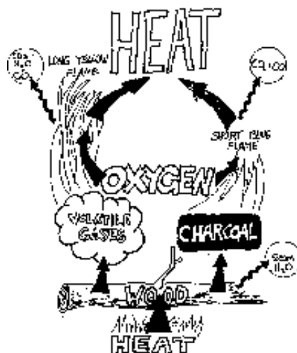
Fig.2-48: Wood burns in two stages. The first, seen to the left, is the burning of the volatile gases. The second, seen to the right, is the burning of the charcoal.
