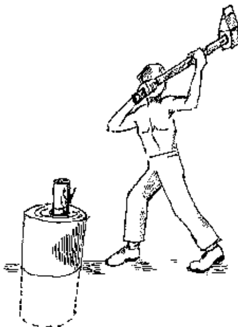
Fig.2-40: a solid chump of wood half-buried in the ground is the proper base for splitting firewood
