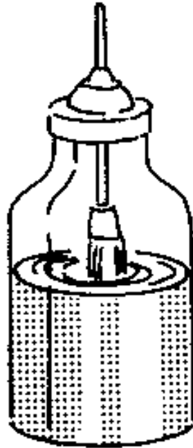
FIGURE 3. A DISPENSER CAN BE MADE BY CUTTING A HOLE IN THE COVER LARGE ENOUGH FOR THE HANDLE OF A 2.5 CM. BRUSH. THE DISPENSER MUST BE AIRTIGHT SO THAT THE CEMENT WILL NOT DRY OUT.
