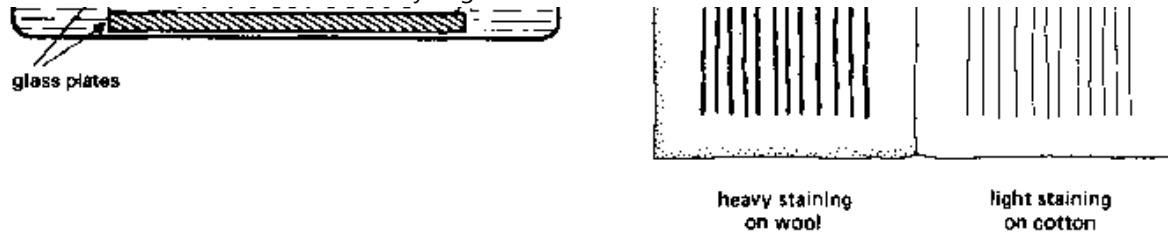
Figure 2: Water fastness testing: loss of colour and staining onto wool and cotton
